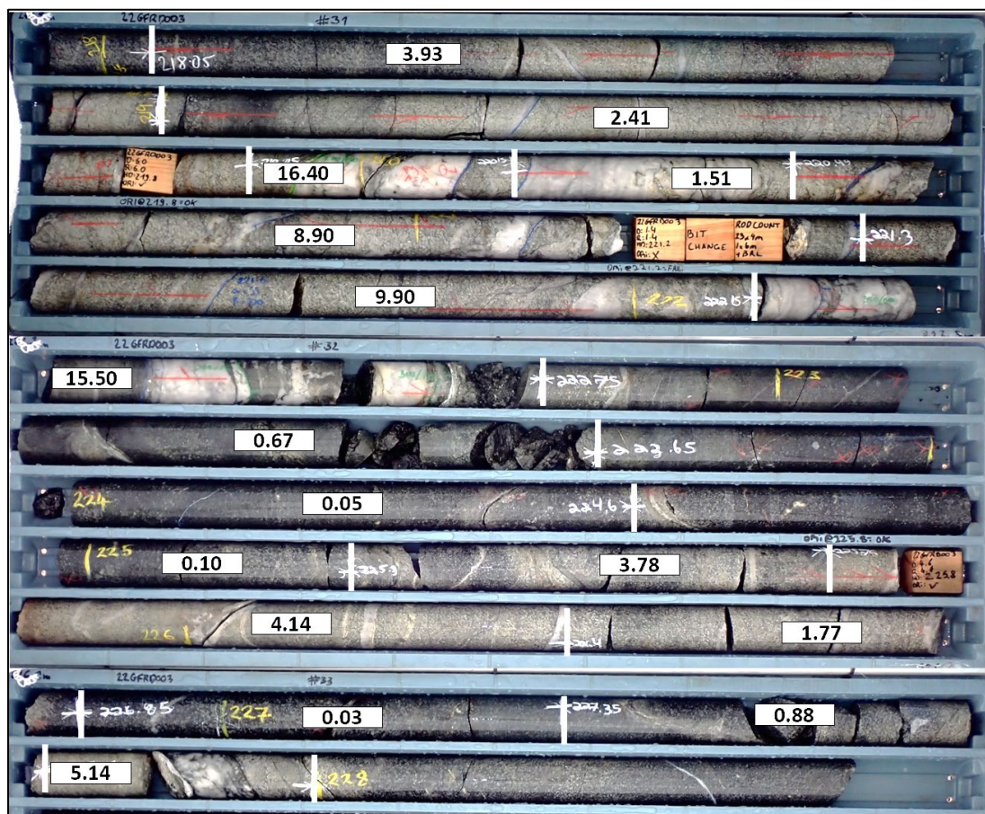
Photograph 1 - Sovereign drill hole 22GFRD003 – 8.50m @ 4.48g/t Au from 218.35m including 4.40m @ 8.01g/t Au from 218.35m (showing assay results in g/t Au). Quartz reef/stockwork hosted in silica-sericite-pyrite altered Great Fingall Dolerite.
