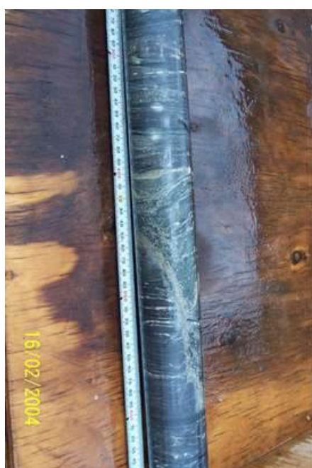
Figure 8-2 Example of the SIF/SIG hosted mineralisation and the steeply dipping north-northwest shear zones in hole WRD04 - Source: Westgold.
