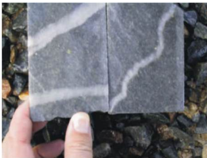
Figure 8-3 Mineralised vein set with disseminated pyrite cuts pervasive north to north-northeast-striking foliation in Cuddingwarra felsic intrusive - Source: Westgold.
