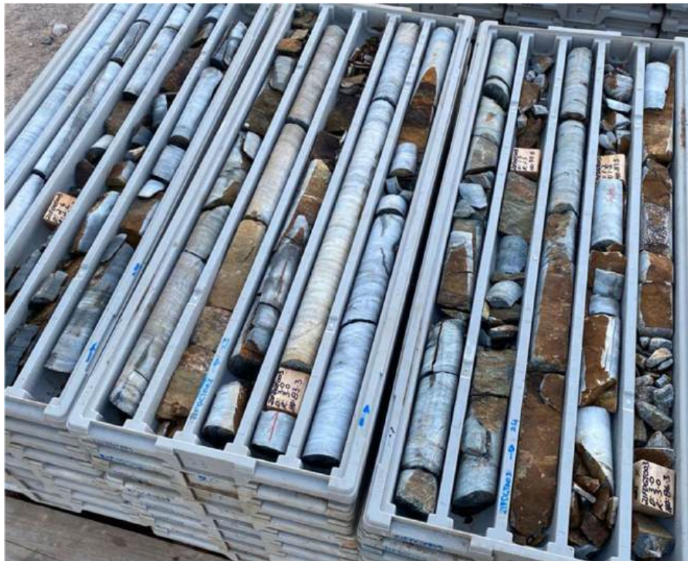
Figure 16-14 Preferentially weathered structures at low angle to the long core axis in hole 21FDGT003. Source: Westgold.
