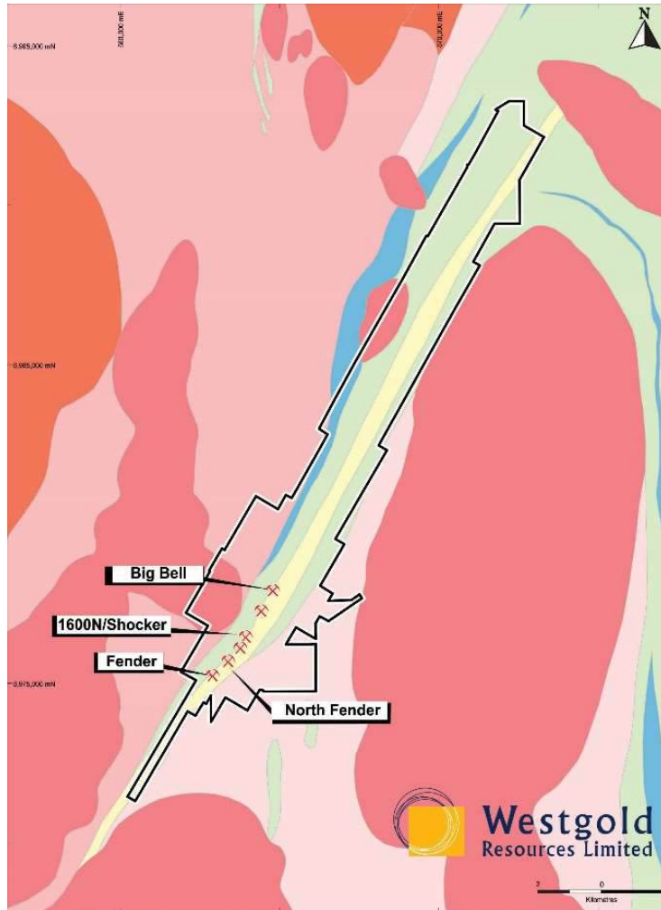
Figure 16-5 Schematic outline of Big Bell area geology showing the Big Bell mine sequence squeezed between the surrounding granite bodies: Westgold.
