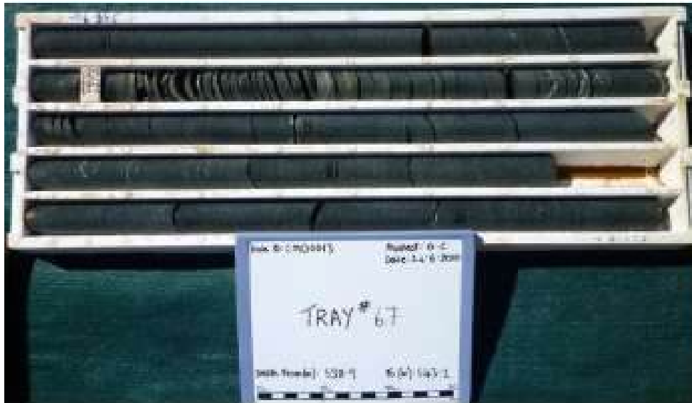
Figure 16-22 Example of intense discing seen in Golden Crown core. Source: Westgold.
