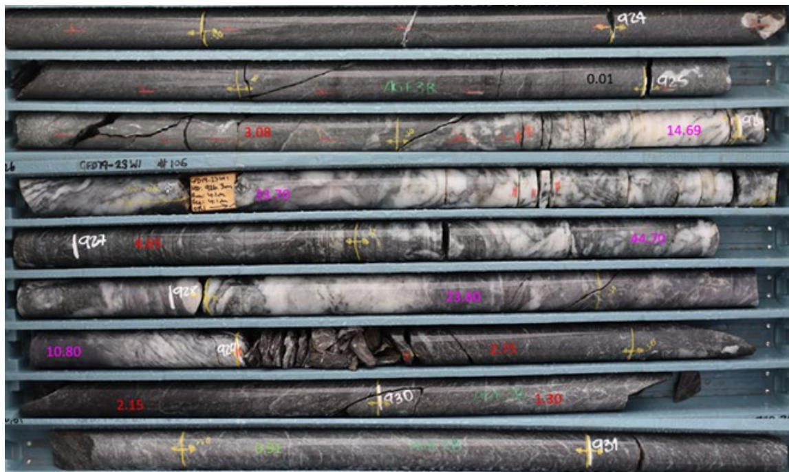
Figure 13 – Lower Fingall Reef In Hole GFD019_23W1 Returned 5.50m @ 16.68g/t Au (Assays Annotated)
