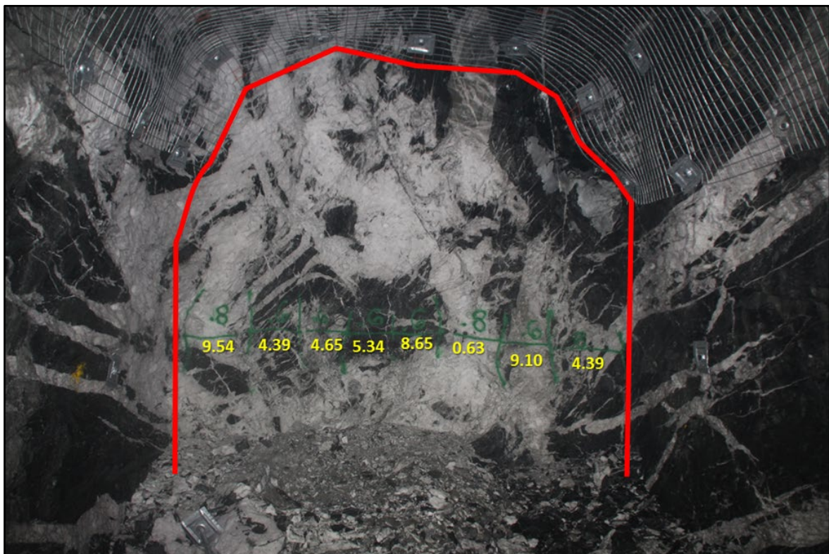
Figure 7-7 Face assays – Western Flanks Central 325NOD1-57 collected (gold grades g/t in yellow, assay interval in green) – Source : Westgold.
