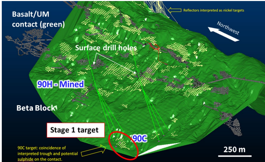
Figure 9-7 3D seismic interpretation identifying high reflectance anomalies interpreted as nickel sulphide. The Stage 1 90C drill target was tested intersecting porphyry intrusives on the basalt-ultramafic contact - Source: Westgold Resources.
