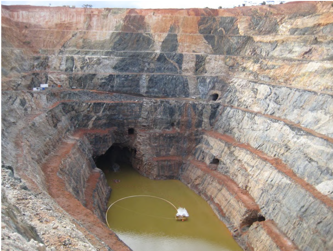
Figure 16-10 North wall of the Chalice pit showing the three main lithological zones, granite, ultramafic and amphibolite, along with various intrusive – Source: Westgold.
