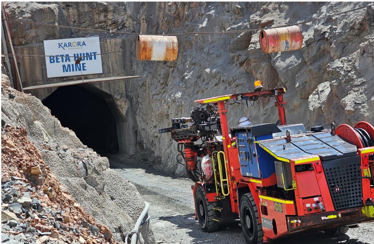
Figure 2 – First of two planned Westgold drill rigs entering the Beta Hunt Portal to accelerate the Fletcher Resource Definition program.
