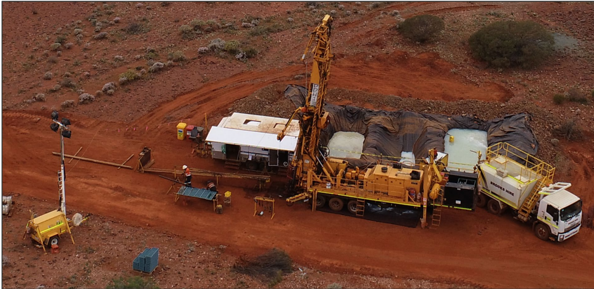
Figure 13 – Diamond Drill Rig On The First Parent Hole (22GFDD006) – October 2022
