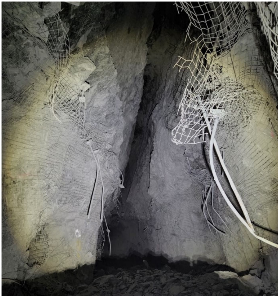
Figure 8 – Example spur stope extraction.
