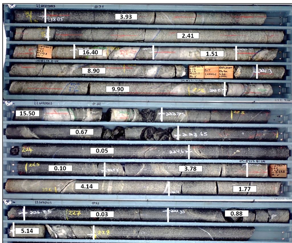
Photograph 1 – Sovereign drill hole 22GFRD003 – 8.5m at 4.48 g/t Au from 218.35m (showing assay results in g/t Au). Quartz reef/stockworks
